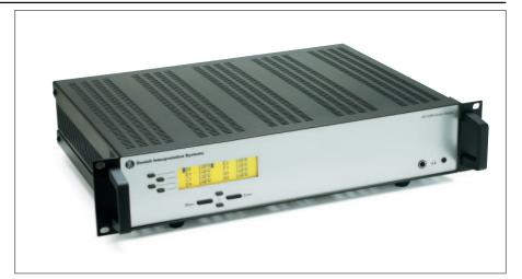
The AO 6008 Audio Output Unit is an 8 channel digital to analogue audio converter designed for the DCS 6000 Digital Conference System. It is used as the D/A converter for analogue language distribution systems, such as infrared orwired transmission systems, tape- or harddisk recorders etc.
